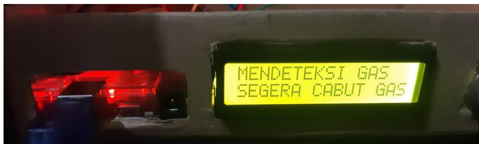
Gambar 7 Tampilan LCD saat kebocoran gas
