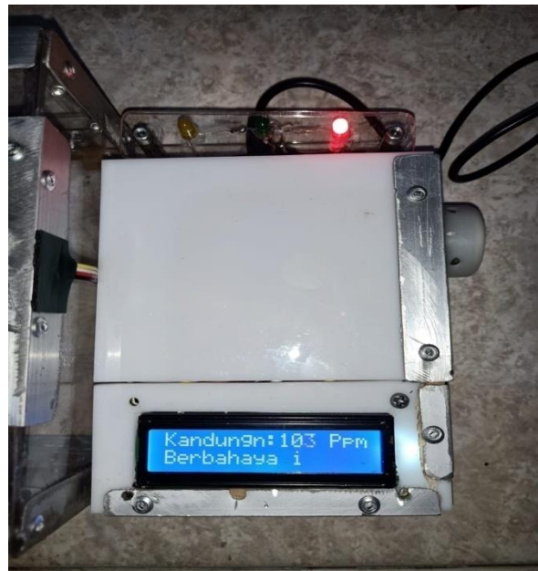
Fig 8 Then the sensor will automatically actively detect formalin in the sample
