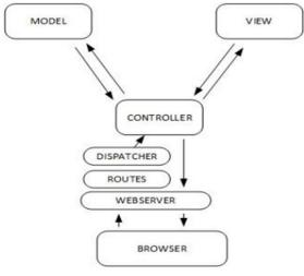
Figure 1: MVC Workflow
